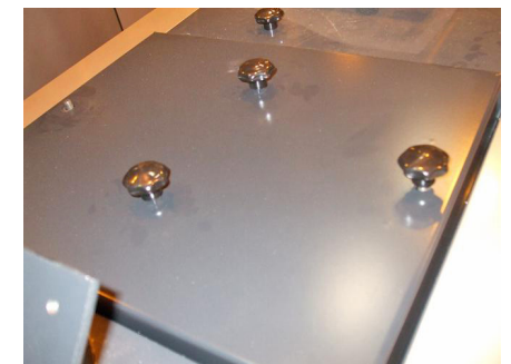
8. Replace the Convection cleaning hatch and fasten the start knobs.
