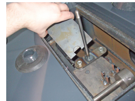
4. Raise the Turbulator lift, remove the Turbulator cover plate.
