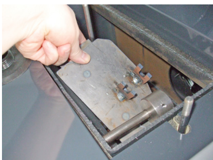
5. Remove the second Turbulator cover plate.
