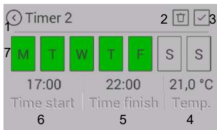
Fig. 60: Creating heating times
