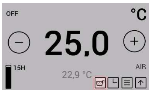
Fig. 86: Riddling grate display
