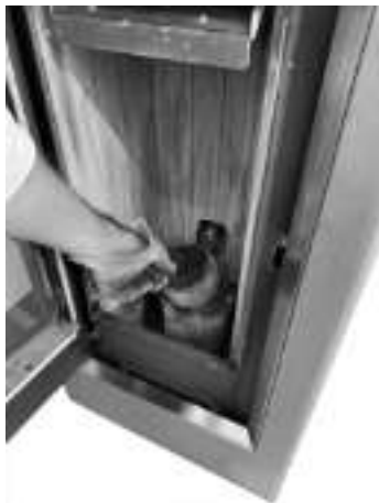
Fig. 31 - Burning pot extraction
