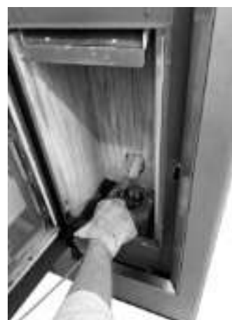
Fig. 34 - Cleaning with a brush
