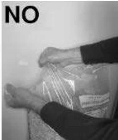
Fig. 22 - Wrong opening of the pellets bag
