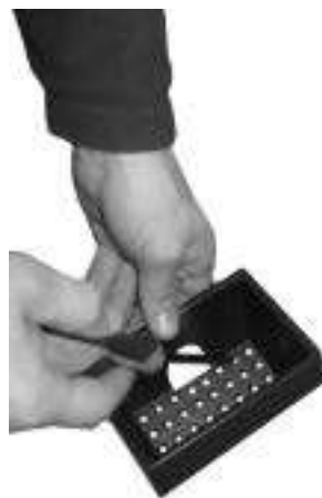
Fig. 33 - Burning pot cleaning
