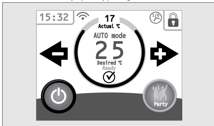
Fig. 3.28 Touch control panel – Child lock
