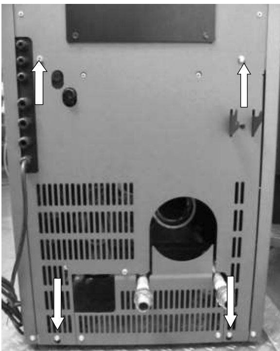
Afb. 88: Demontage bekleding modellen Pat, Frank, Dave, Ray en Jack
